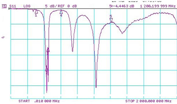
Figure 2 illustrates a typical PIFA S11 where deep resonances represent high efficiency. There is room for improvement at 300 and 600 MHz; however the antenna is seen to operate well in switchgear.
