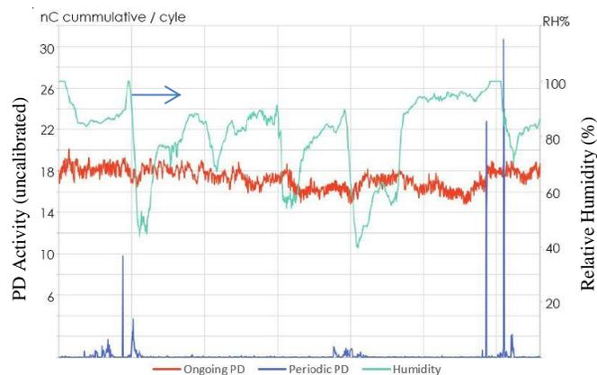
Figure 10 illustrates long-term corona activity in the 300 MHz band and abrupt PD and corona activity in the 1200 MHz band. Abrupt activity correlates to saturating humidity.
