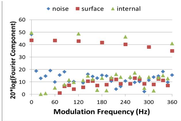
Figure 4 illustrates the DFT content for a 60 Hz line frequency when presented with noise, surface, and internal discharge signals.
