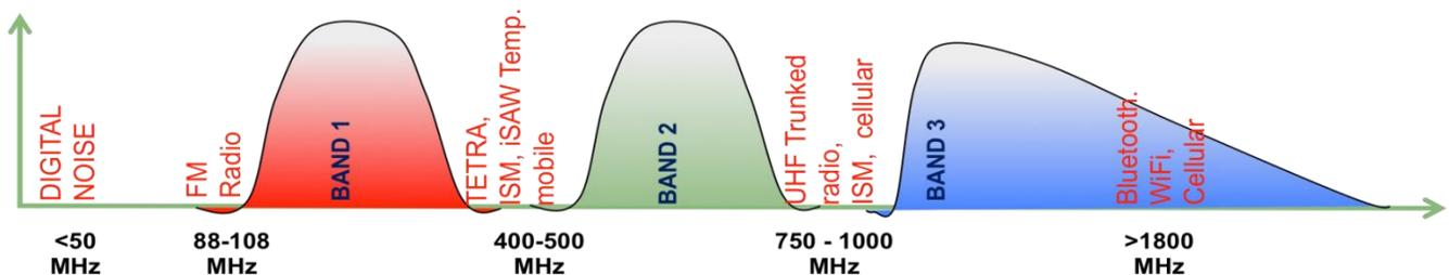
Figure 1 illustrates the three bands selected for the UHF detector and the various known interfering signals to be filtered.
