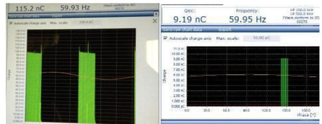
Figure 5 illustrates the response of a PD Smart in direct measurement mode for a PD synthesizer having no resistor (left) and 20K $\Omega$  (right).
