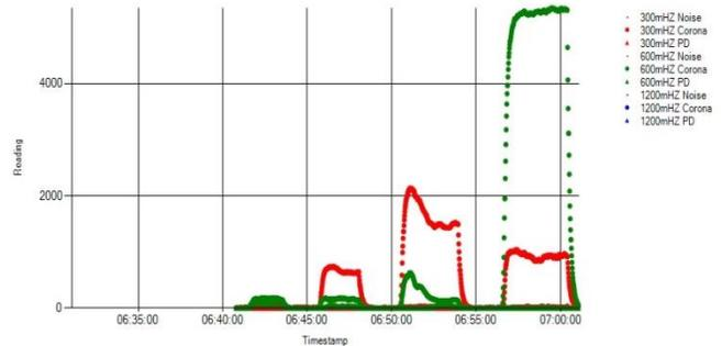
Figure 8 illustrates the response to 15kV applied through normal insulation distances and then reduced to sub-standard spacing.
