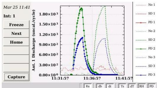
Figure 7 shows a screen capture of the 600 and 1200 MHz responses to synthesized PD and Corona discharges in a 22 kV GPT.
