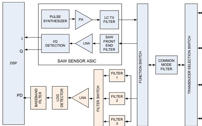
Figure 3 shows existing SAW sensor measurement subsystem (blue) and added electronics for PD monitoring.
