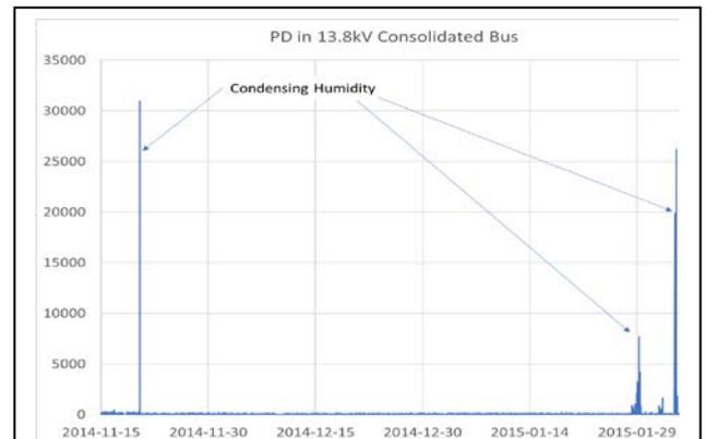
**Large PD events in a distribution substation with inadequate humidity control. Dew point rated spacers had no accumulated damage.**
