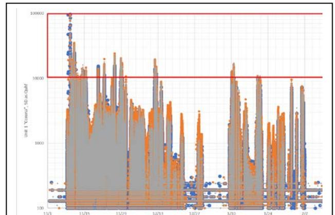
**Large PD events in a generator iso-phase bus duct during start-up resulting from dust after major construction.**
